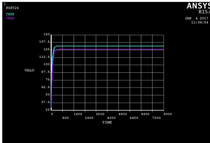
*Fig. Response time or time to reach steady state for aluminium material*
