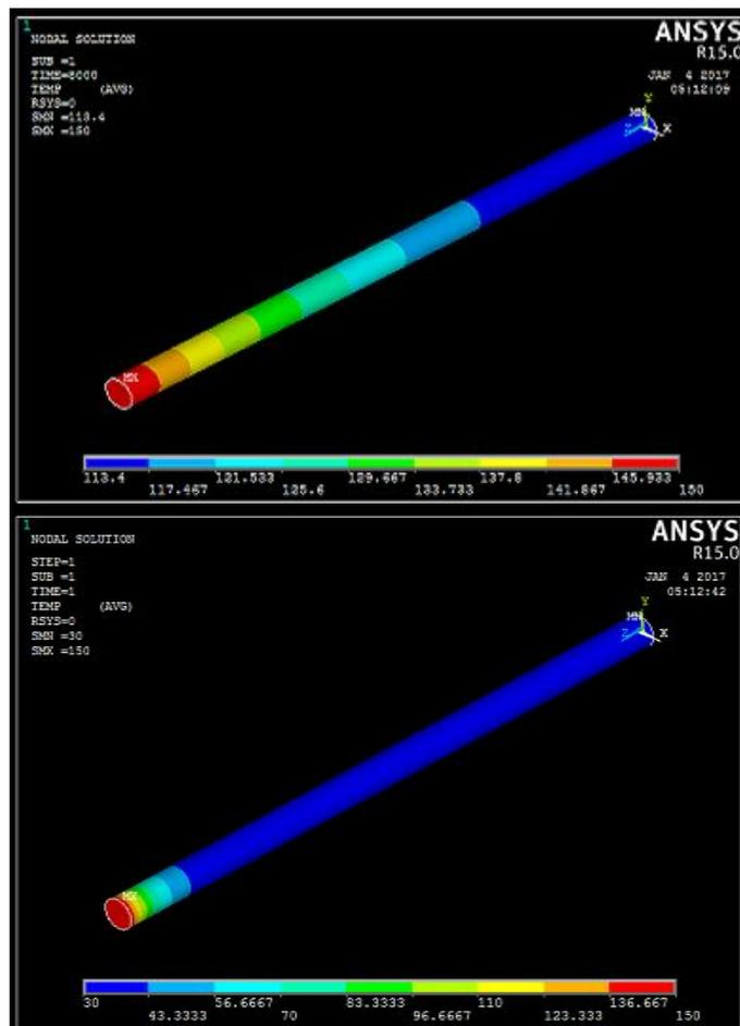
*Fig. Temperature distribution at 8000 seconds for brass fin in Transient Analysis*
