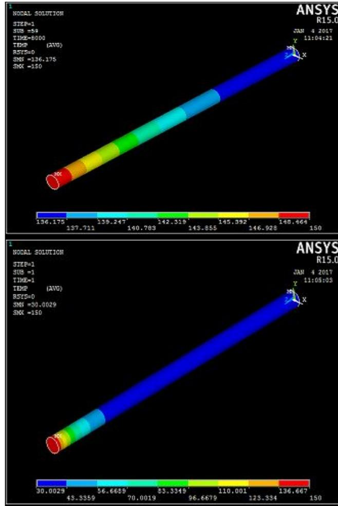
*Fig. Temperature distribution at 8000 seconds for copper fin in Transient Analysis*
