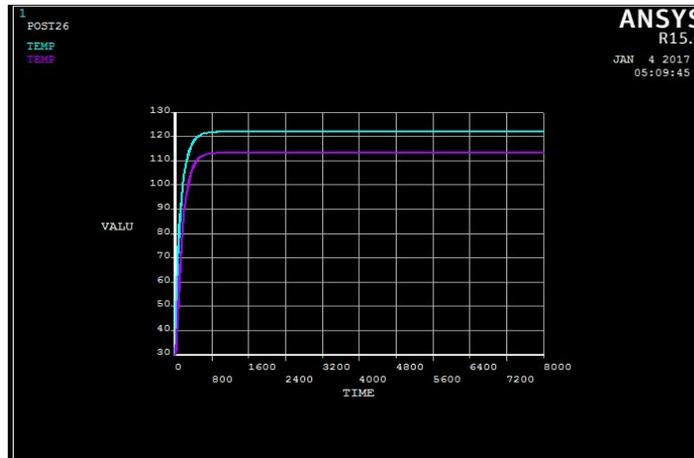
*Fig. Response time or time to reach steady state for brass material*
