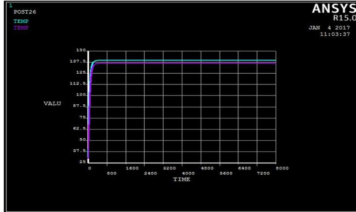
*Fig. Response time or time to reach steady state for copper material*
