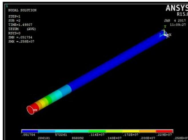
*Fig. Heat flux (W/m<sup>2</sup>) variation for copper fin material*
