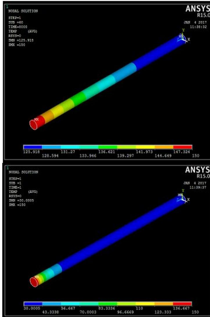
*Fig. Temperature distribution at 8000 seconds for aluminium fin in Transient Analysis*
