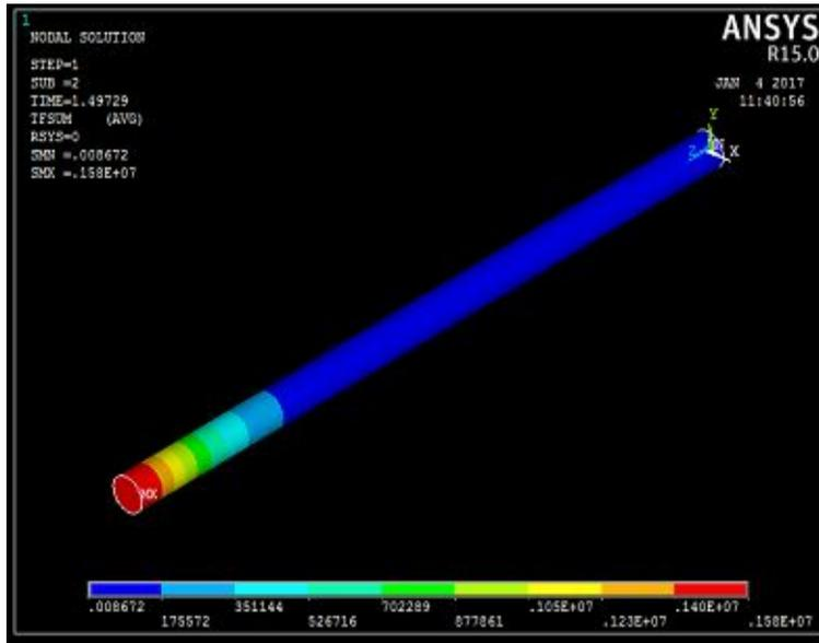
*Fig. Heat flux (W/m<sup>2</sup>) variation for aluminium fin material*
