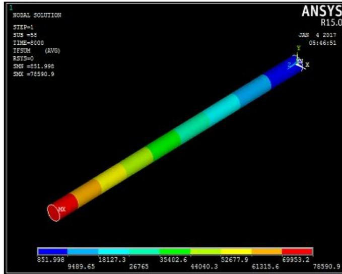
*Fig. Heat flux ( $W/m^2$ ) variation for brass fin material*
